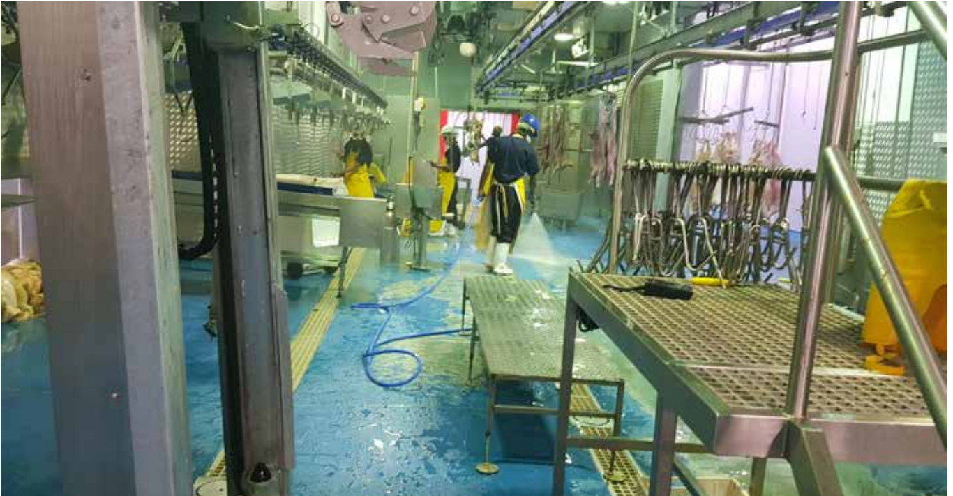
FIGURE 7: MANUAL CLEANING LOW FLOW SYSTEM
