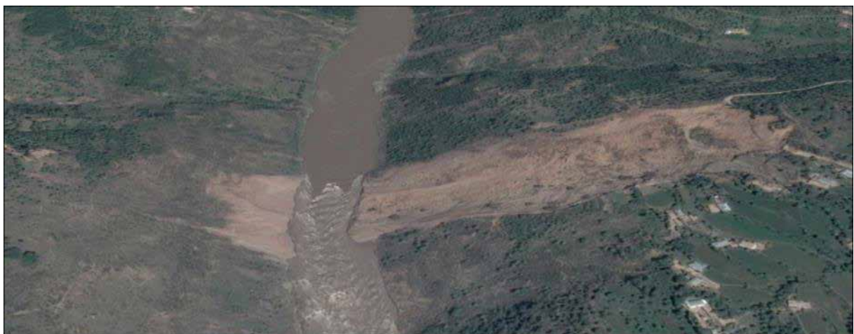
Figure G.A.12: Google Earth Image of a Landslip Altering the Flow of the Lower Jhelum River about 35 km Downstream of Muzaffarabad
