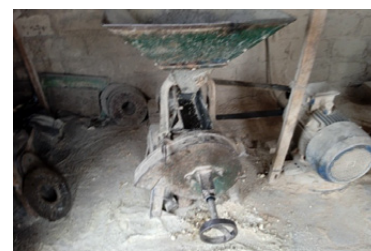
Picture 3. Small maize miller (grinder)
