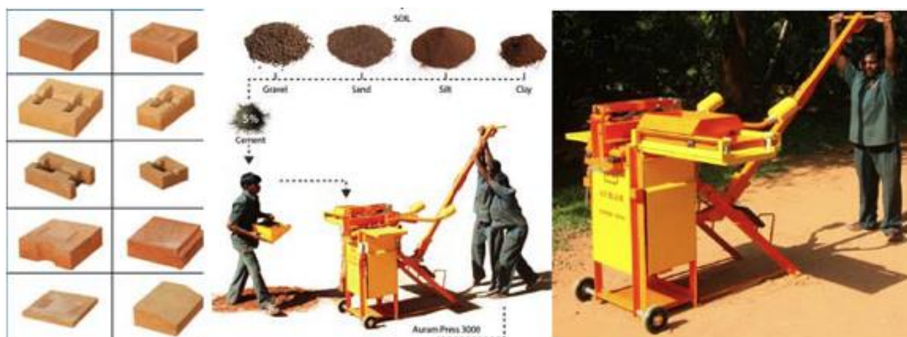
Figure 33: Composition of Compressed Stabilized Earth Blocks (CSEB)
