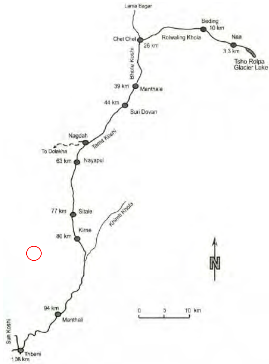
Figure 20. Geographic delimitation of the impact of the Tsho Rolpa Glacier Lake outburst (up to 100 kilometers downstream). The red circle represents the discharge point of Khimti Khola hydropower plant on the Tama Koshi (about 80 kilometers of the lake).
