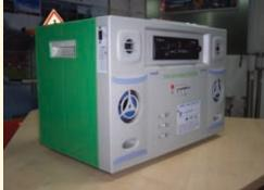
**Beijing Sunpu** developed a new Solar Home System "plug and play" unit built of durable plastic. The plastic casing gives the PV system an attractive appearance and provides room for including a radio, VCD or DVD player, and speakers. Two casing sizes have been developed—one for small systems (10–30 Wp) and one for larger systems (30–60 Wp). The total project cost was Y 572,000 (US\$77,000), with a CG Facility grant of Y 150,000 (US\$20,000).
