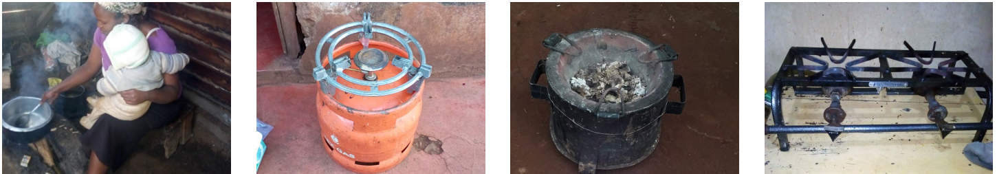
From left to right: Three-stove fire, an LPG stove, a Kenyan jiko stove that burns charcoal and a Sistema.bio biogas stove. Source: Eco Consultancy & Research Ltd.
